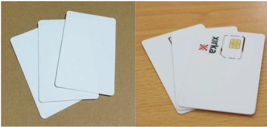
Gambar 1. Chipset Smart Card (Kiri: Contactless Card, Kanan: Contact card dan SAM)
